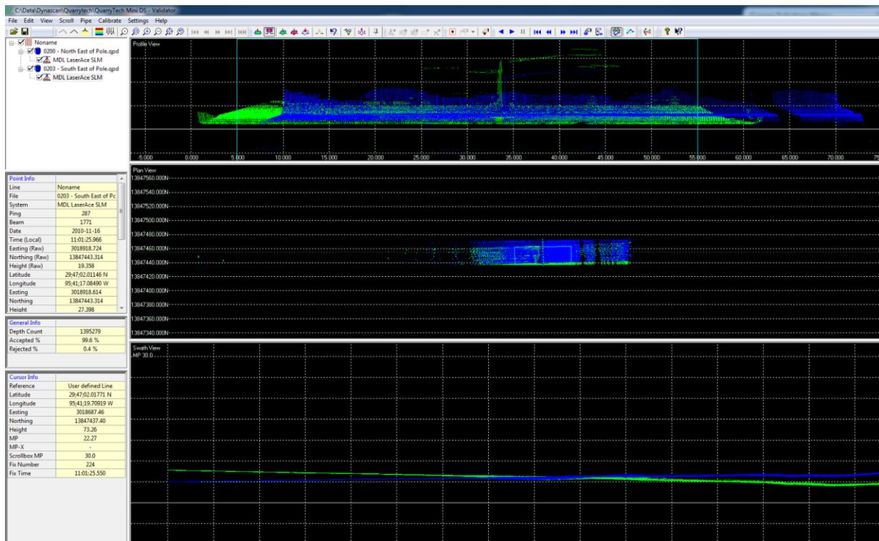
9. Make the slice box fit the flat area where the two files were recorded.
