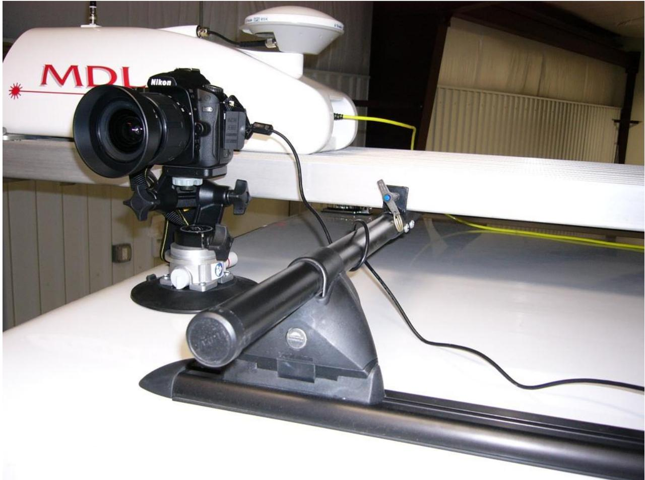
The picture below shows the USB cable connected between the camera and laptop computer running QINSy. USB extension cables will be required to extend the Nikon supplied cables.
