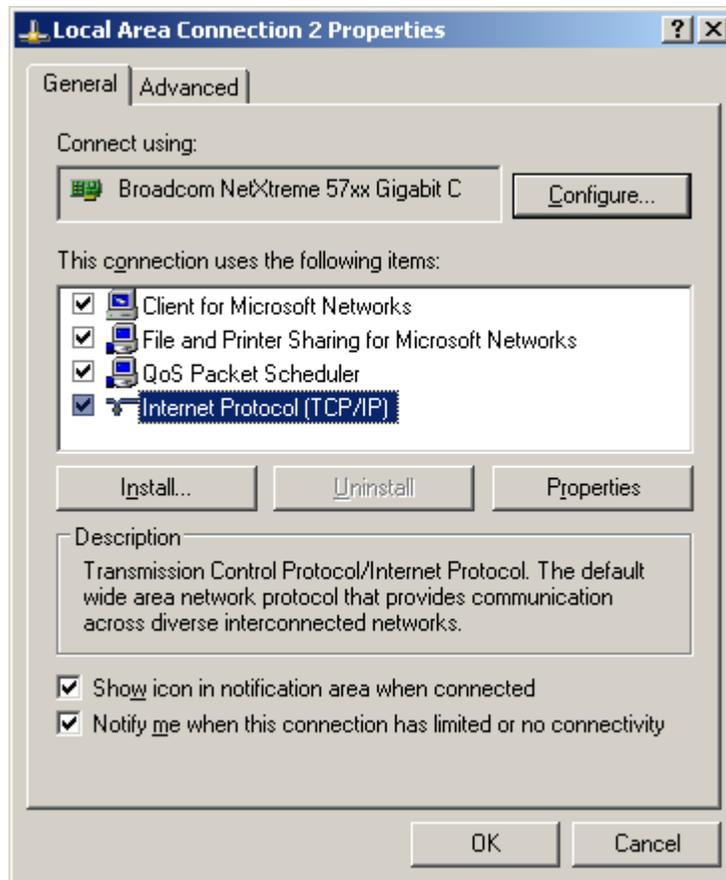
The IP address entered here is slightly different than the laser IP address, an example of which is shown below. The system will not work if this number is exactly the same as the laser IP address.
