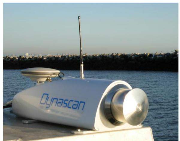
It is important to line up the pod and secondary GNSS antenna along the centreline of the vehicle (see photo below). Try to fabricate brackets / fixing holes for the pod and secondary antenna so that the system can be re-installed in the same place. This will save time, as you will not need to re-calibrate the heading.
