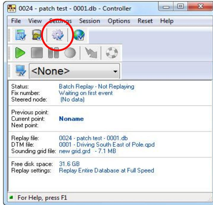
Select sounding grid and modify any settings, as required and then click on the DTM File button.
