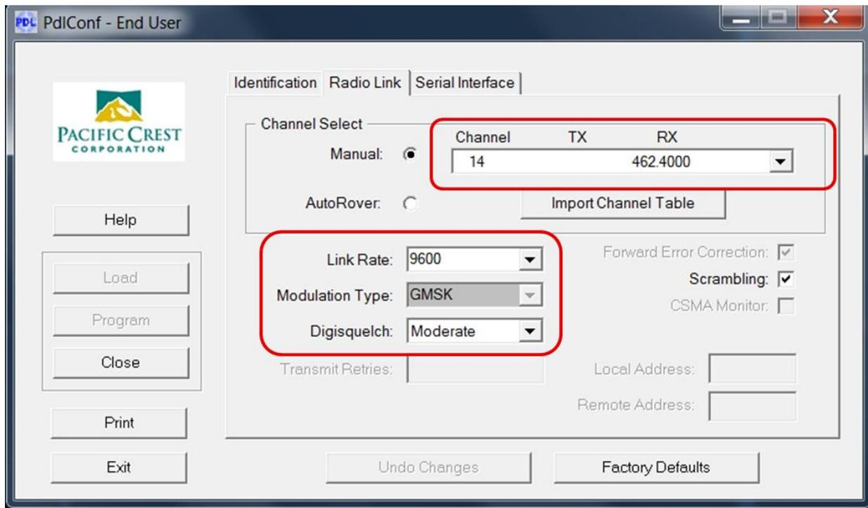
Confirm that the Radio Frequency, Link Rate and Modulation Type are compatible with your GPS RTK Base Station.
