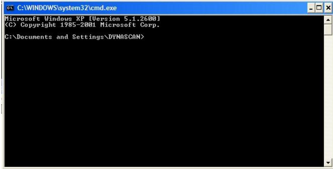
Ensure the IA is switched on before typing **ping 128.2.0.201** and then enter (using the IP address of the Dynascan unit, which is on a label underneath the unit and also shown on the QINSy setup page).
