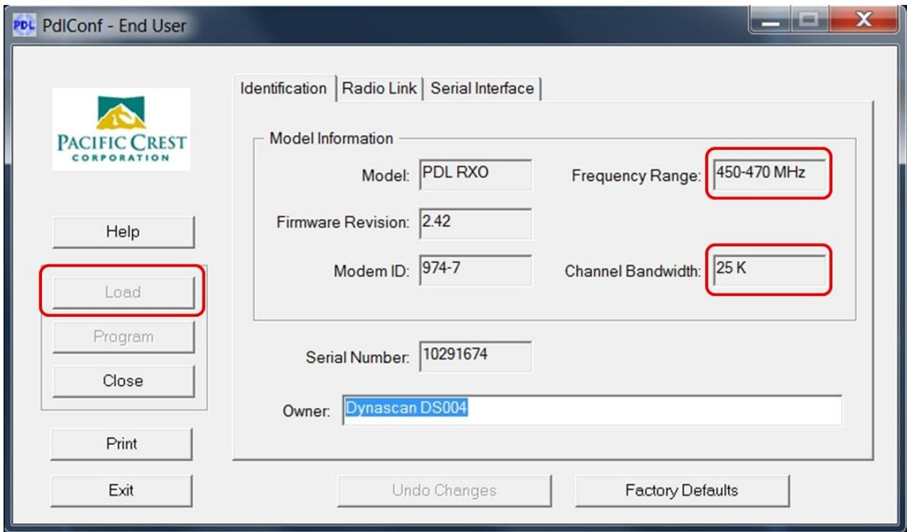
Once you have loaded the Radio settings confirm that the Frequency Range and Channel Bandwidth are compatible with your GPS RTK Base Station.
