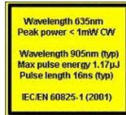
**WARNING –Visible and invisible laser radiation. Do not stare into the beam.**
