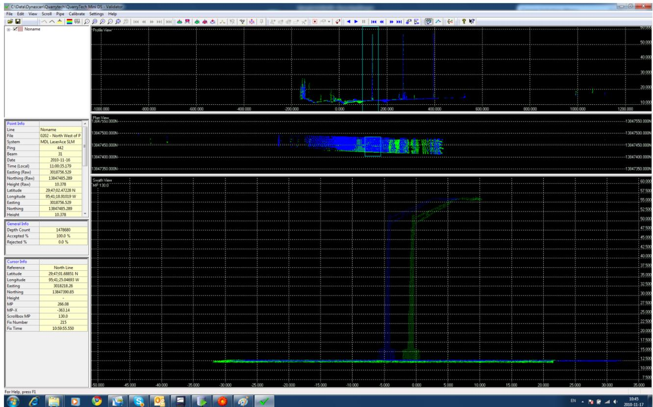
25. You will see that the two images are parallel but not aligned and so you must click the View=Validate icon and then the Calibrate Alignment icon to bring up the values box.
