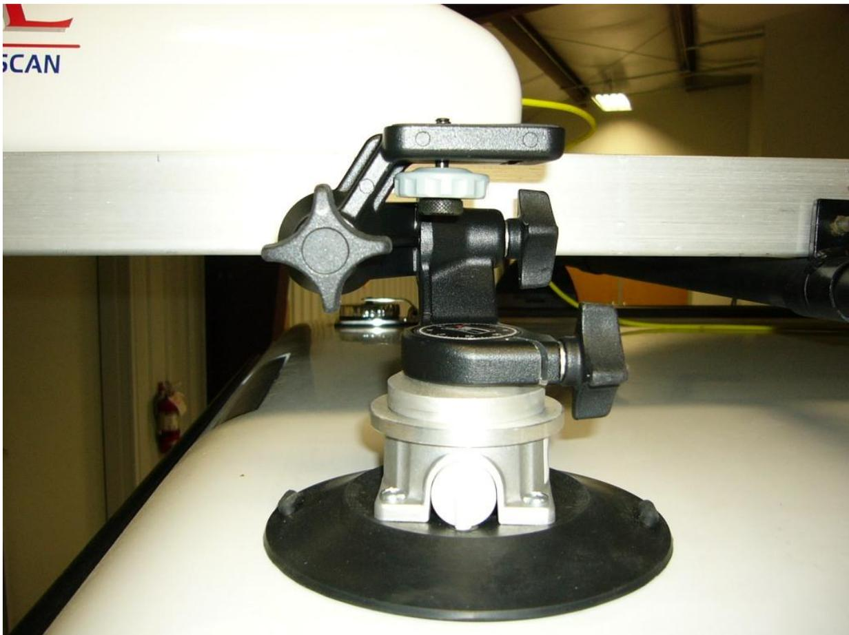
**N.B. If using suction caps use a lanyard, or the camera strap, to tie the camera to the roof rack as a precaution against the camera falling.**
