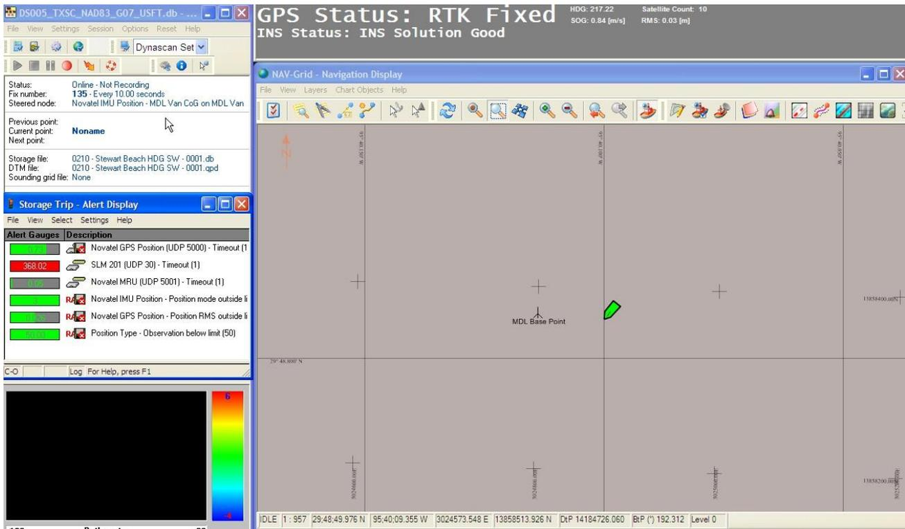
You should now only have one red alert in the Alert Display, which is the Laser alert (SLM). Click on 'settings' and select echo sounder settings then click the control tab and switch on the laser next to the scanning box.
