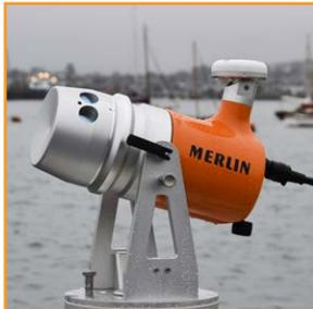
The custom-made mounting plate ensures rapid installation and deployment.
